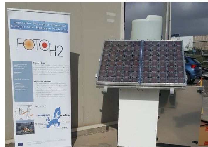
FotoH2 Panel Glass Electrode Membrane Assembly (GEMA) concept
