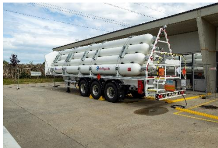
Trailer: Air Liquide (200bar, ~300kg H 2 )
