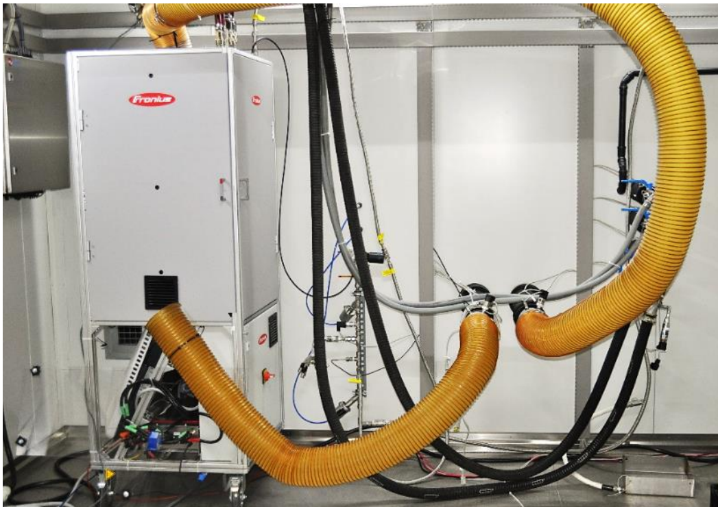
Figure 4-3: Set up of fuel cell system on the fuel cell system testbed Schönbein at HyCentA
