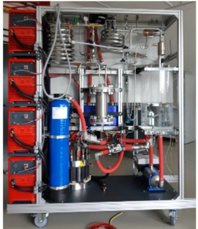
Figure 3-21: CAD drawing and ready assembled prototype of PEM electrolysis system
