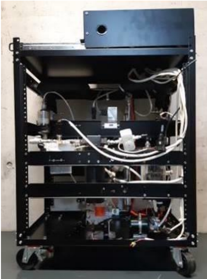
Figure 3-12: Electrolysis single cell test station
