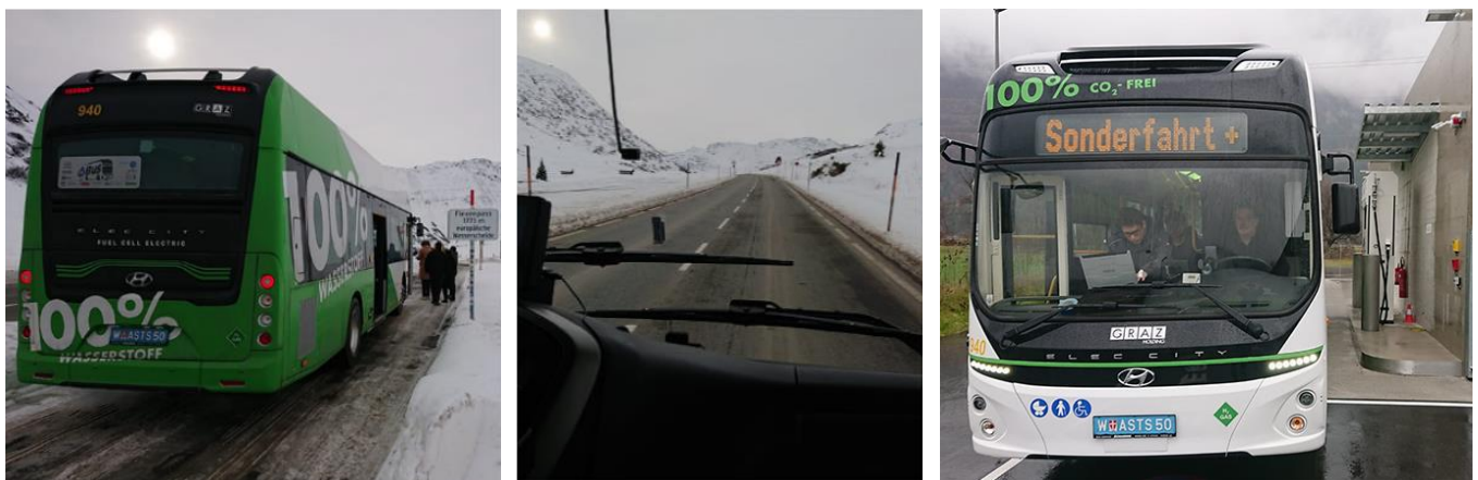
Figure 14: Test drives with Hyundai Elec City FCE hydrogen bus from Holding Graz within the HyBus R&D project, Source: Hyundai Import GmbH; Refuelling the Hyundai ElecCity with green hydrogen at the MPREIS HRS (source: Hyundai Import GmbH).
