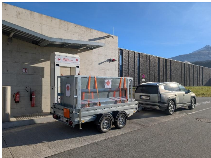
Figure 16: Novel Backup & Emergency Hydrogen Logistics System especially for small scale applications.
